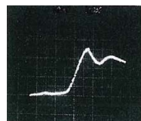
Figure 2: Analogue ESD measurement
